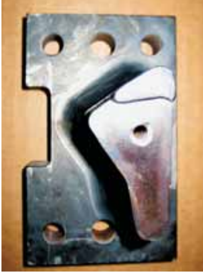
Weld restoration of D-2 metal-stamping punch
