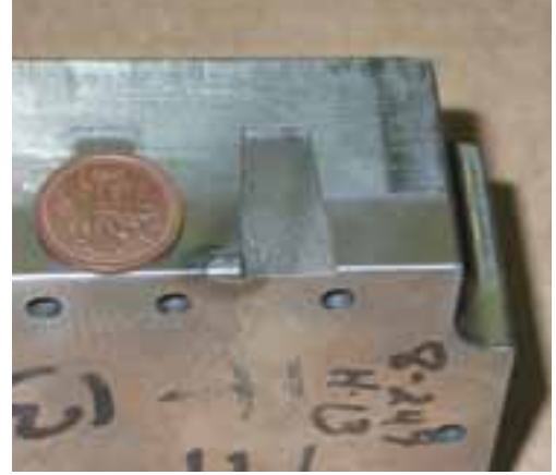
Micro TIG repair using 0.007" wire on an H13 injection mould block
